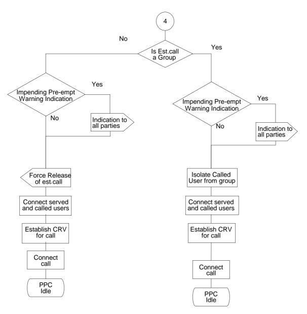
Figure 1 (sheet 3 of 3): SS-PPC supplementary service, overall SDL
