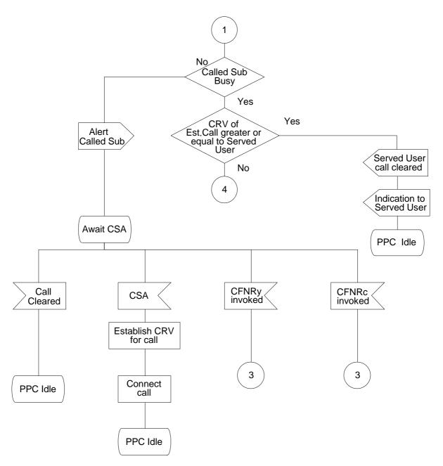
Figure 1 (sheet 2 of 3): SS-PPC supplementary service, overall SDL
