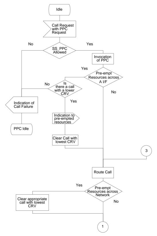
Figure 1 (sheet 1 of 3): SS-PPC supplementary service, overall SDL
